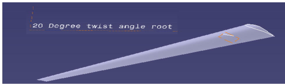
Figure 18. Catia v5 3D cad Modal with single blade 20° twist angle at root
