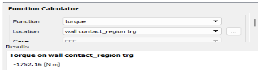
Figure 10. torque results at 5 m/sec air velocity and standard air blade design
