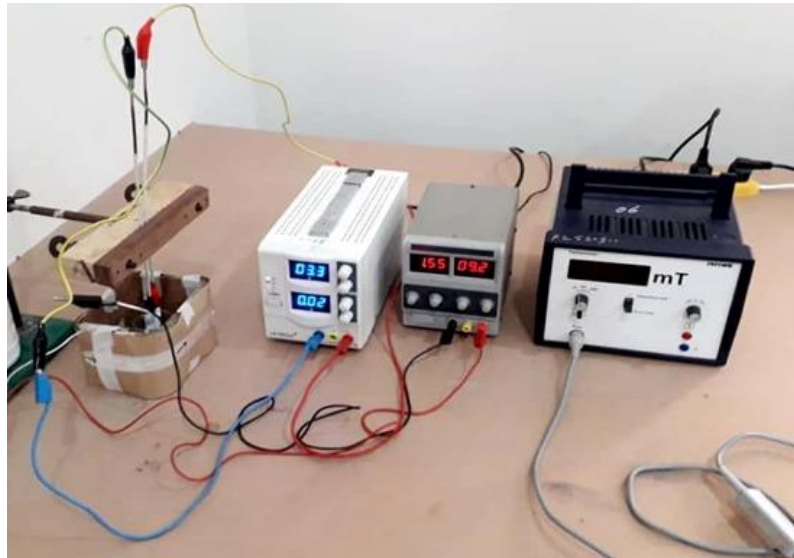
Fig. 2: Apparatus setup for electrochemical deposition
