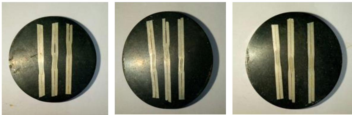
Fig. 8 Mould of a sample after polishing and moulding process
