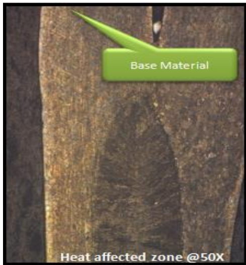
Fig. 19 and Fig. 20 Microstructure for weld zone and heat affected zone for sample 7 At 50X magnification
