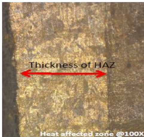
Fig. 13 Microstructure of weld zone for sample 2
