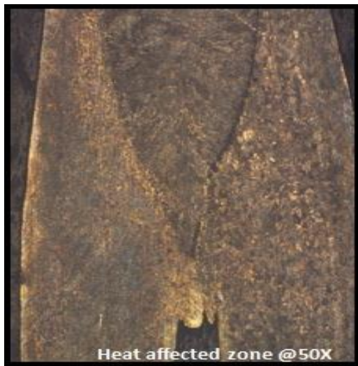
Fig. 21 and Fig. 22 Microstructure for weld zone and heat affected zone for sample 8 At 50X magnification
