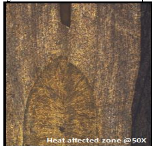
Fig. 16 Microstructure of weld zone for sample 5
