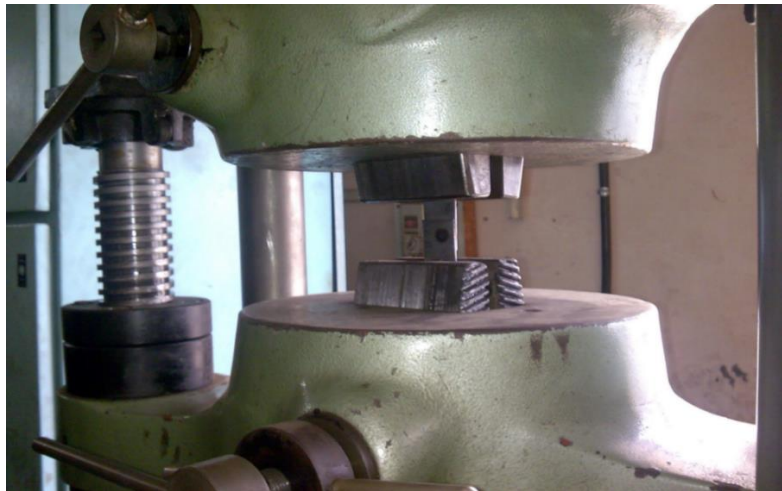
Fig. 7 Clamping of specimen on UTM
