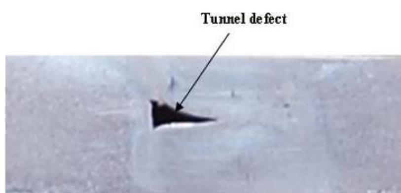
Fig. 3. Defects in welded workpieces prepared at tool rotation speed of 1100 rpm.
